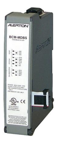
The BCM-MDBS is a BACnet-compliant gateway to a Modbus EIA-232, EIA-422, or EIA-485 network. The BCM-MDBS is a fully programmable network controller. It hosts its own schedules, calendars, alarms, trend logs, and DDC.
