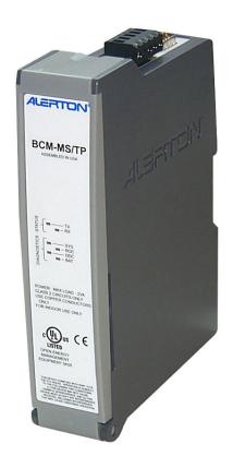
The Alerton® BCM-MS/TP is a high-performance global controller that supports up to 65 field controllers on a single BACnet MS/TP LAN. MS/TP is a LAN standard designed specifically for BACnet applications using the EIA–485 signaling standard on twisted-pair cabling in a simple bus configuration.
