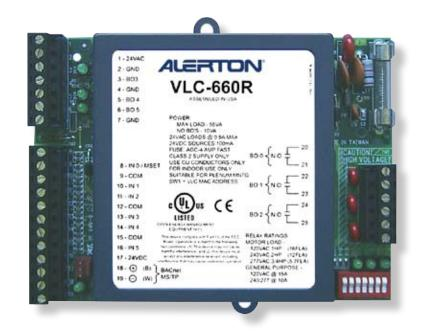
The Alerton<sup>®</sup> BACtalk<sup>®</sup> VLC-660R is a versatile, fully programmable BACnet-compliant field controller. With three software-controlled highcurrent relays, the VLC-660R is well suited for unit ventilator and fan-coil applications, or any application that requires multi-speed fan or motor control. As a native BACnet controller, it integrates seamlessly with your BACnet system, communicating on a BACnet MS/TP LAN at up to 76.8 Kbps.
