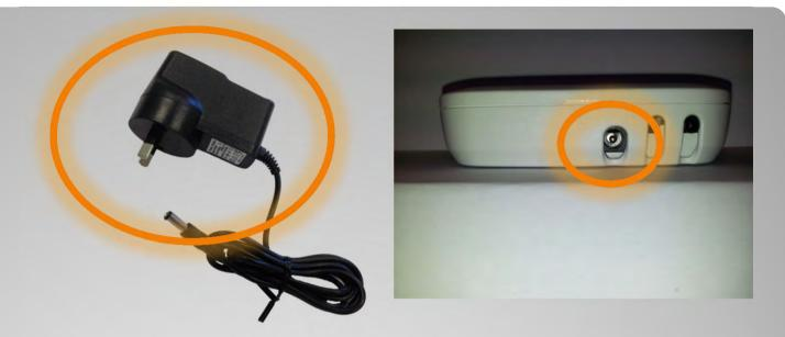
Using the supplied low voltage transformer, plug your Pebble into a local electrical socket.
