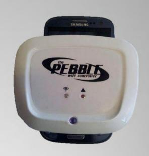
Plug in the Pebble, press the "Send BlinkUp" button and immediately place the pebble on top of the screen of your smartphone, as shown above
